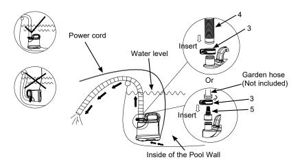
**NOTE:** Maximum pool **water depth** not to exceed 48 in (1.22 m). To protect the pump motor from running dry, disconnect the power cord from the electrical outlet once the water has been drained out or when the remaining water is below the drainage pump base.
